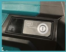
Full sequential actuation mode for single nailing
