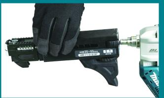
New and improved casing attachment allows for quick attachment/removal reducing the trouble of reversing and replacing a bit
